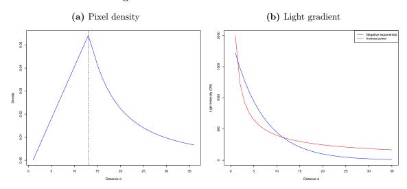
Notes: The left panel shows the pixel density from eq. (4) with  $x_c=10000$  and  $\phi=1.5$ . The right panel shows the negative exponential distribution with  $\gamma=0.15$  as well as the inverse power distribution with a=0.7, both start at  $P_0=2000$ .
